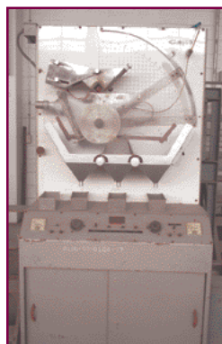
High Tension Separation
